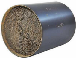
90603282 Diameter= 93mm Length= 130mm 200cps(Cells) / Euro4
