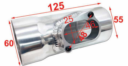
AG-262PP \Phi 60 L125 Thickness=1.5mm Suzuki Swift 1.2/1.4 '2010-Up ZC32S, ZC72S, ZC82S
