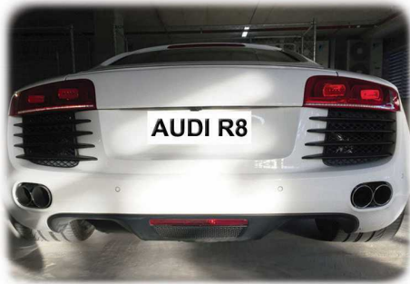
152377-03 S/Steel-Chrome plated Audi R8 V8 4.2L Dimensions=2x89 IN=190x110 Fits the OEM bumper
