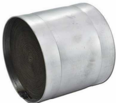
SUB1140 Diameter= 120mm Length= 110mm Euro4 / 400cpsi(Cells) For engines up to 3.0L
