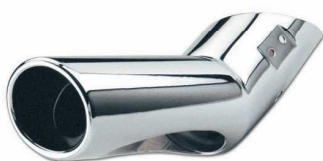
06-8502 S/S-Chrome plated M/des W163 ML320/ML350 Total Length=285mm Oval=120x80 Inlet(ID)=70mm
