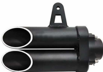
TR007AA Aluminum Inlet Diameter=50mm, BD=2x60mm Body Length=280mm / Double Layer
