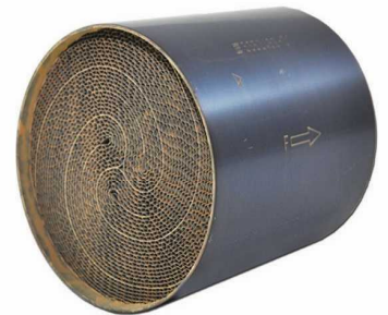
90603244 Diameter= 121mm Length= 110mm 200cps(Cells) / Euro4 HF+ (For High Temperature)
