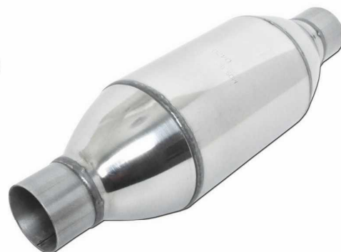
C12 Inlet=60mm, Body Diameter=127mm Total Length=420mm Metallic substrate 200cps / Euro4 Designed for performance road vehicles
