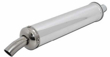
TR037A-S S/Steel / ALUMINUM Inlet Diameter=25mm, BD=60mm Body Length= 300mm
