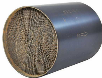
90603250 Diameter= 108mm Length= 130mm 200cps(Cells) / Euro4 HF+ (For High Temperature)
