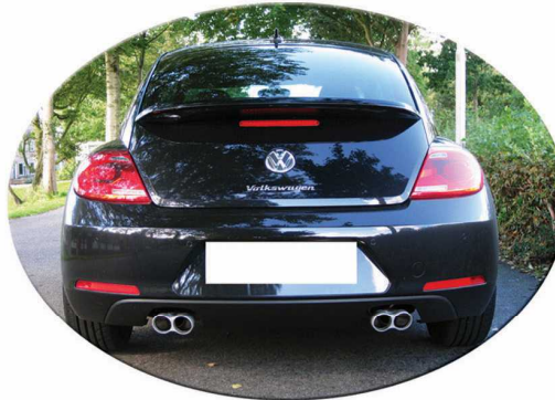
152181-01L (Left) 152181-01R (Right) 149x74 L200-175 INΦ64 Single layer / S/Steel with Aluminium endings
