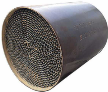
90603297 Diameter= 130mm Length= 130mm 100cpsi(Cells)
