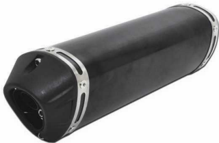
TR041A-BK (Black Paint) S/Steel / ALUMINUM / MATERIAL ABS TR041A-CC (Carbon Look) S/Steel / ALUMINUM / MATERIAL ABS Inlet Diameter=38mm, BD=100x90mm Body Length=300mm / DB Killer
