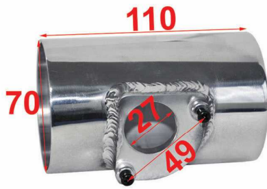
AG-016PP \Phi 70 L110 Thickness=1.5mm HONDA CIVIC 2.0 08-09
