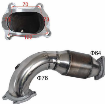
DP10 S/Steel Down pipe \Phi 76 for FIAT ABARTH: 1.4T 500 (135hp/160hp) '2008- 1.4T 595 Turismo/Competizione (160hp) '12- With HJS racing Metallic Cat 200cpsi Doesn't fit on the OEM system
