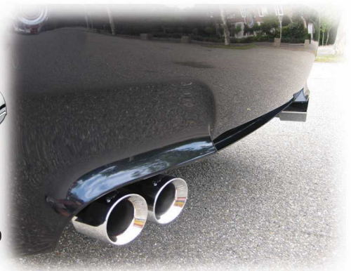
06-7720SL/R L225-185 \Phi 76 Slant & Side Slant IN \Phi 60 S/Steel+Chrome plated 'Ferrari style'
