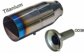
21089 S/Steel-Titanium Total Length=210mm Diameter=89 Inlet(OD)=60mm Includes a removable DB Killer
