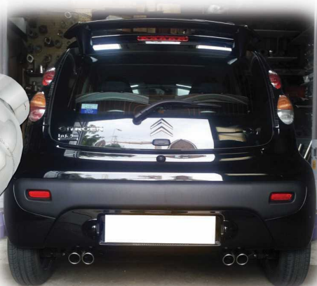
BL217L (Left) BL217R (Right) L200-190 2x \Phi 60 IN58 Slant Cut / Double layer For Toyota Aygo/ Citroen C1/ Peugeot 107
