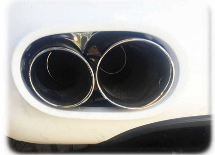
152377-05 Carbon Audi R8 V8 4.2L Dimensions=2x89 IN=190x110 Fits the OEM bumper
