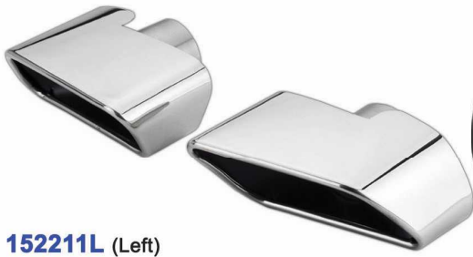
152211L (Left) 152211R (Right) 176x74 L155 INΦ60 «AMG W212 E350-E500» Look Double layer / Chrome plated
