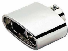
06-5603S S/Steel T304 BMW 318i E36 '90-'00 BMW 520i E34 '89-'97 Total Length=160mm Oval=155x75 Inlet(OD)=64mm
