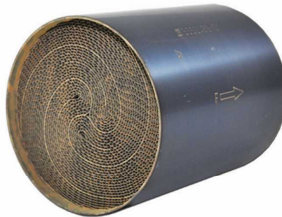
90603295 Diameter= 130mm Length= 130mm 200cps(Cells) / Euro4 HF+ (For High Temperature)
