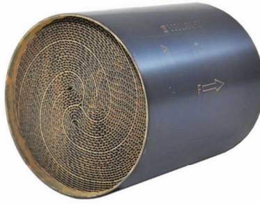
90603340 Diameter= 121mm Length= 130mm 200cpsi(Cells) / Euro6
