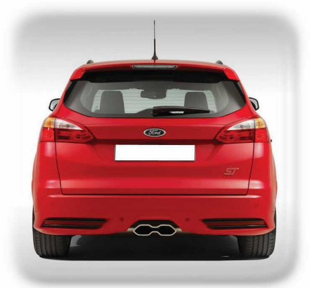
152838 S/Steel-Chrome Plated Ford Focus ST Style Total Length=240mm Dimensions=275x75mm Inlet(OD)=64mm
