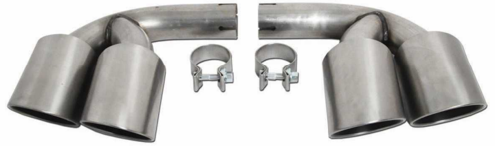
TR-3697 (Left & Right) 2x102 L360 Slant & Side Slant INΦ60 Porsche Cayenne 9YA Turbo '2017+' Brushed Polished
