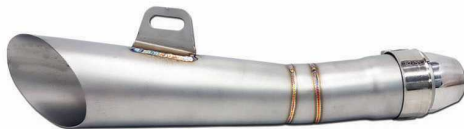
TR016SS S/Steel Inlet Diameter=50mm, BD=76mm Body Length=350mm / DB Killer
