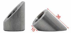
LB040 Mild Steel Lambda boss with 40dgrs angle M18 \Phi 27 L=36-10mm
