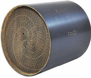
90603347 Diameter= 108mm Length= 100mm 200cpsi(Cells) / Euro5 HD (For Porsche and High Performance Cars)
